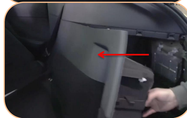
3. Pry the trim panel cover on the right (the same operation on the left)
