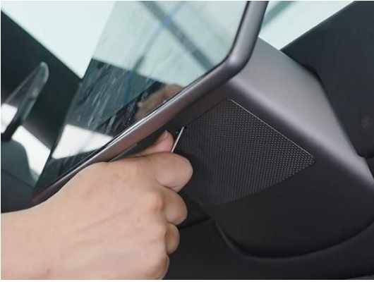
9. Remove the lower cover under the center control screen
