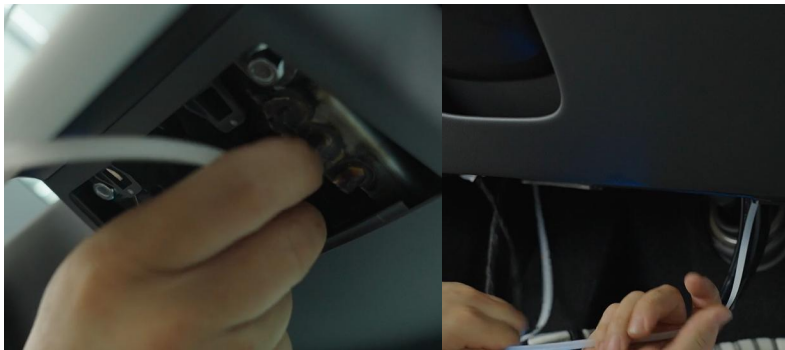
11. Pass the harness from the screen bottom to the driver's footwell
