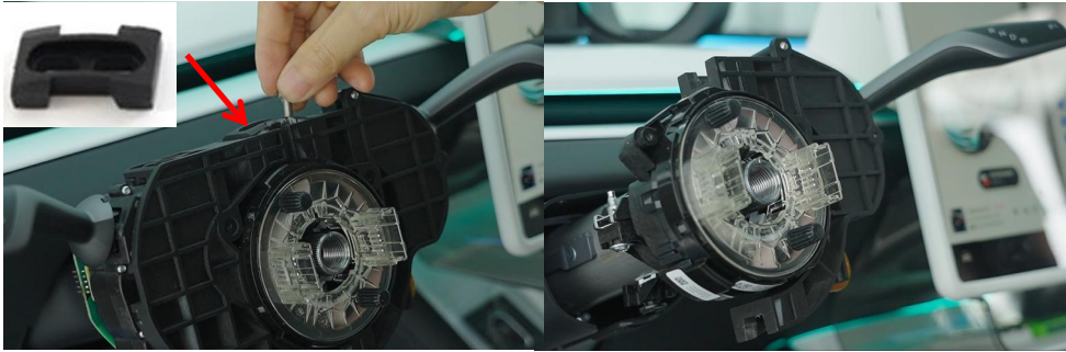
5. Install the gear shift stalk and use the ⑤ fixing gasket and provided screws to keep it in place
