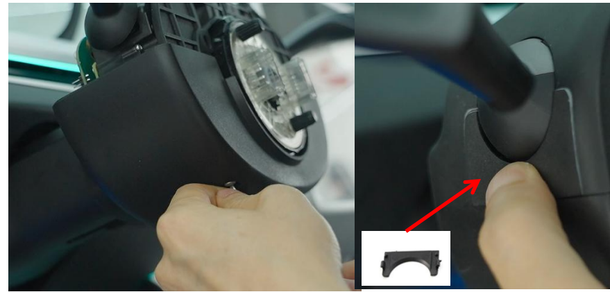
14. Install the upper and lower covers and put on the small cover
