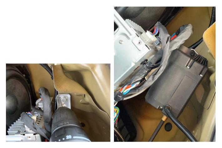
The cable between the motor and catching hook must be put behind the carpet. Release 2 clips to do so.
