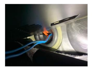
Use a piece of sturdy electrical wire to pull the + of the power cable (part 9) through this hole, so it enters the frunk area. Use this wire to pull the + connector of the power cable through. Connect the connector in the plug of the fuse holder.
