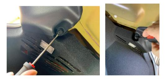
The lower part can just be pulled up. Than pull the carpet on the left and right sides inboard, and remove the cable from the trunk flood lights.
