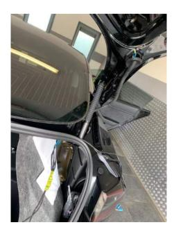
When you managed to get the wire in the trunk area, get these 2 cables from the liftgate wiring harness (part 10)
