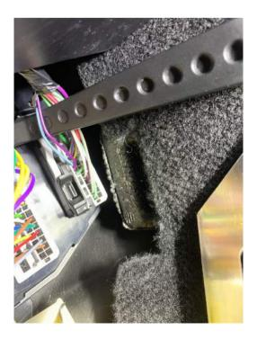
Take the can bus wire (part 8), with the 2 wiretaps already installed, and connect them. The red-white (H) wire must be connected to the blue wire. And the red-yellow (L) wire must be connected to the purple wire.
