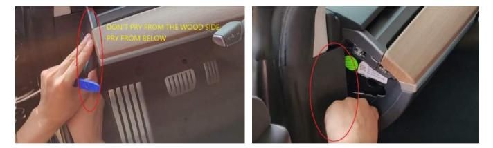
After you removed these panels you can see a clip, from which you need to pop the center first. Than you can pull the doorsill out.
