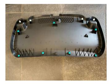
Remove the trim pieces on the top and lower part of the inside of the trunk. For the top piece you first need to remove 2 clips. To remove these clips, you need to pop the inner part with a screwdriver, then you can remove them by hand.
