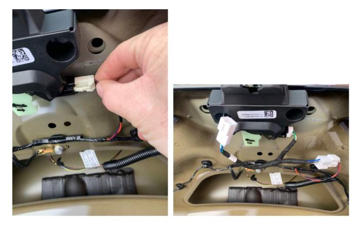
The purple lead from the new harness will be connected with a wiretap to the green wire of the existing switch to open the trunk.
