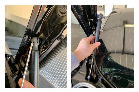
The news struts can be clicked in place easily, without releasing the clips. Be careful to mount the struts with the cables on the bottom, and the strut with the long cable left, and with the short cable on the right.
