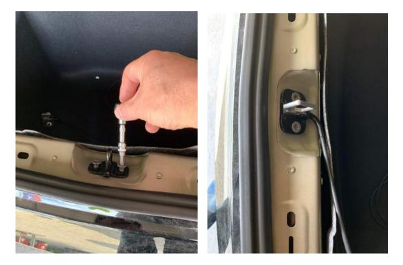
In the bracket where you installed the ground wire, drill a 3 mm hole. This is a good place to install the motor of the motorized catching hook with 1 screw.
